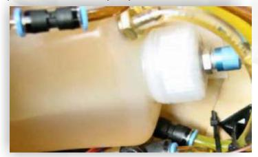
Clear tubing helps identify and locate any potential future problems with air leaks.
